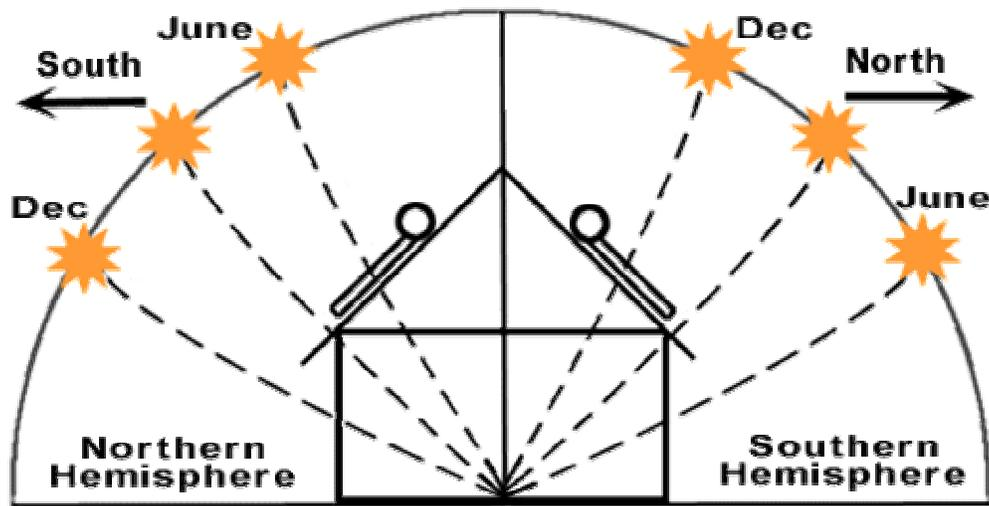
The angle at which you mount the collector should roughly correspond to the latitude of your location. For example:
